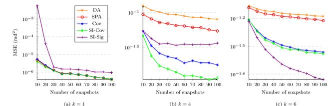
**Figure 2:** MSE vs. number of snapshots. The proposed SI-Cov outperforms Cov, showing the advantage of using the scale-invariant strategy.
