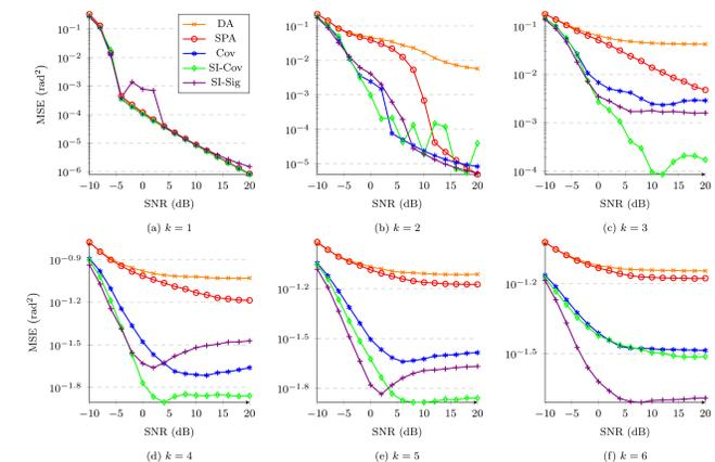
**Figure 1:** MSE vs. SNR. The proposed scale-invariant covariance matrix reconstruction approach (SI-Cov) outperforms DA, SPA, and Cov when  $k > 2$ .
